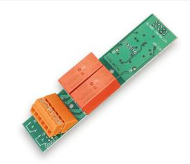
The WM-CUB combines with the RAK8-MB to provide a centralised lighting control system that can integrate with either wireless or wired Rako products.
